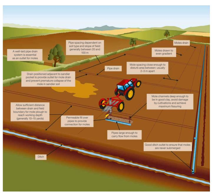
Figure 35. Layout of piped drainage and mole drains
