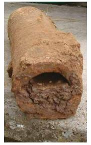
Figure 22. Silted clay drain
