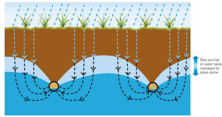
Figure 2. Water table control on permeable soils
