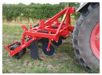
Figure 11. Topsoil loosener for grassland
