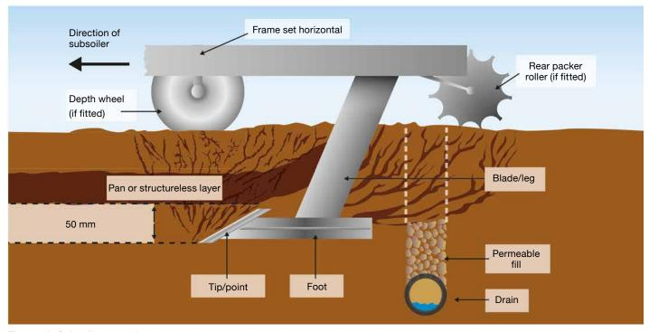
Figure 13. Subsoiler operation
