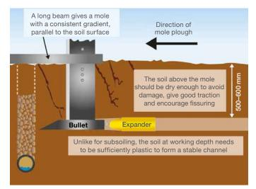
Figure 26. Appropriate conditions for forming mole drains
